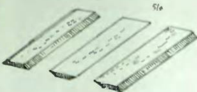
Fig. 51a. Some professionals skive the top edge of the strand on one side, and then skive the opposite edge underneath, while others skive both sides on the top (the beginner may find this the easiest way).
