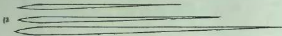
Fig. 12. The second method is to cut out three small pieces of flexible leather. Give them a heavy coating of fat or leather dressing.
