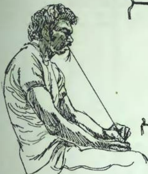
Fig. 92. In this sketch he was using full-length tail hairs. A more usual length would be around 450 mm. The hairs are twisted until they begin to kink.
