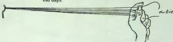
Fig. 94. Wrap some twine around a hook and tie the ends. The length will be about 400 mm. The number of strands will depend on the thickness of the material. If using binder twine you may have to split it into half thickness.
