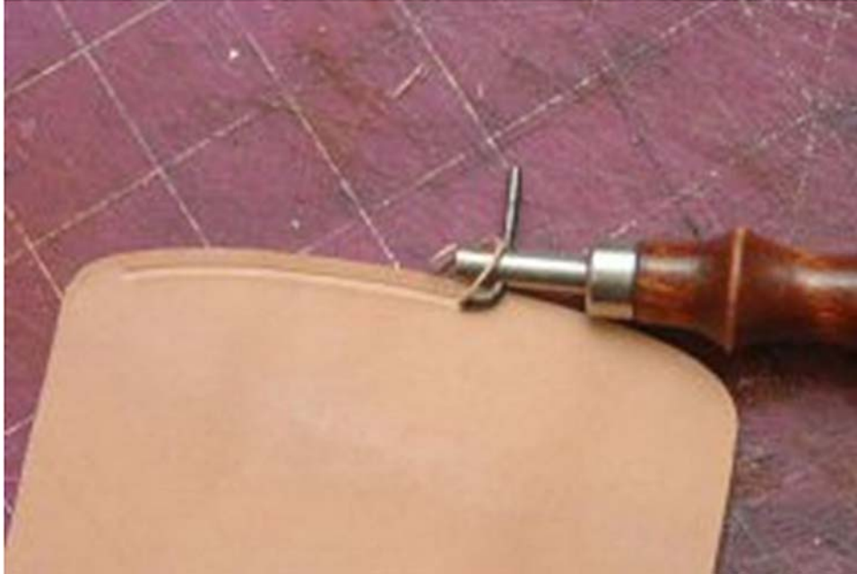
Figure 6: Cutting Stitching Groove
