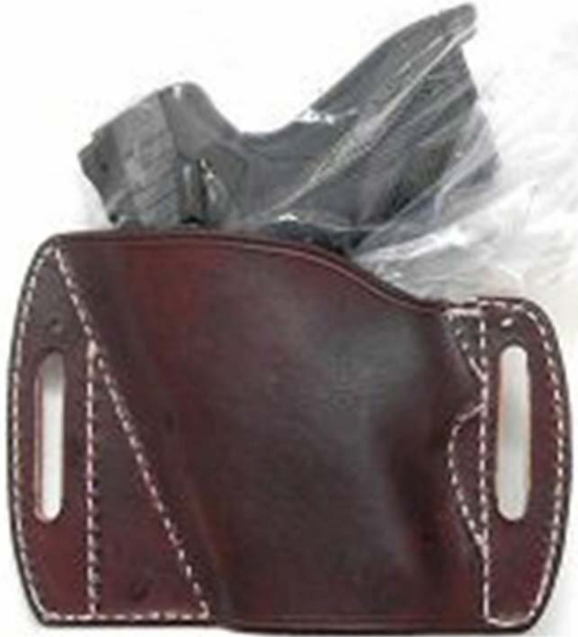
Figure 16: Wet Molding the Holster (shown from the left side)
