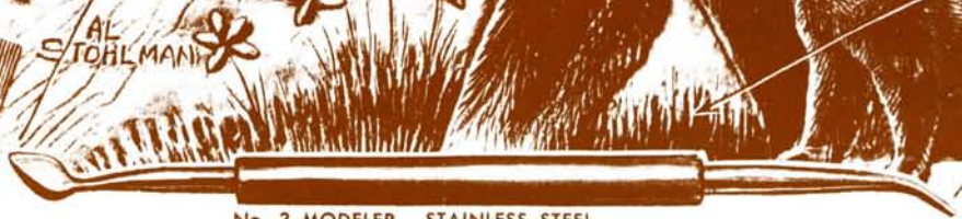
No. 3 MODELER STAINLESS STEEL Used for rounding figures, smoothing rough beveling, forming eye-balls, adding facial expressions and other fine details.
