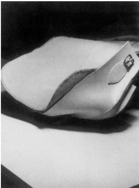
Fig 172 First stitch to join back and flap panel to gusset.
