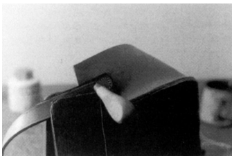
Fig 158 Awl insertion for stitching strap to gusset.
