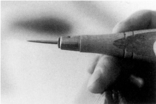
Fig 6 Stitching awl, to show flattened area of handle in line with flat part of diamond-shaped blade.
