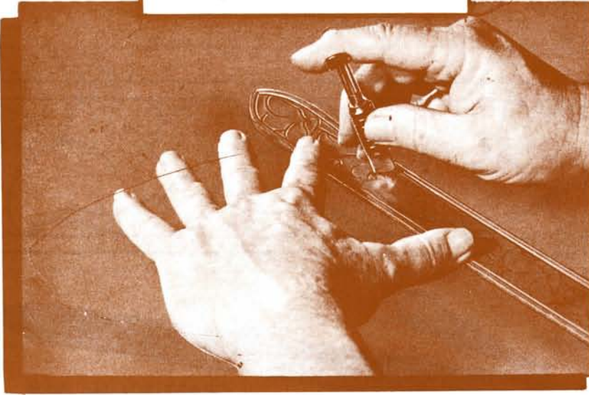
Fig. 3 Begin the carving at the tip. Cut the outlines of the flower, then the stem, leaf, etc. until the full length of the belt has been cut. Turn the leather when necessary to make the free flowing cuts. Never try to cut with the hand in a cramped position. Keep the blade sharp!
