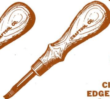
CRAFTOOL No. 8076 Edger For rounding belt edges.
