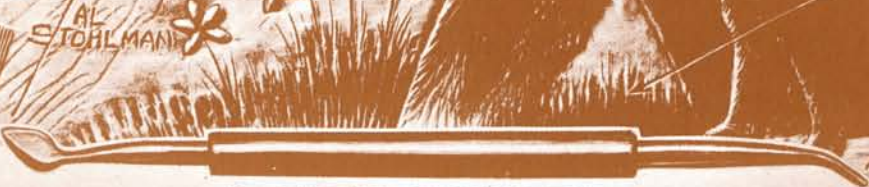
No. 3 MODELER STAINLESS STEEL Used for rounding figures, smoothing rough beveling, forming eye-balls, adding facial expressions and other fine details.
