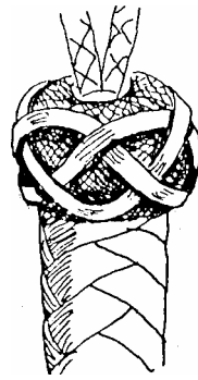
Fig.60. The Turk's-head is spread around the knob like this.
