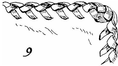
Fig. 9. When going round a corner go through the same hole 2 or 3 times to get a good cover. Remember that corners get the most wear.
