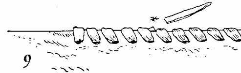
Fig.8. Tighten up the lacing and then pull the end tight. If you have pushed the end between the two pieces of leather then pull it tight from the inside.
