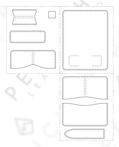
Once EACH 8"x10" dashed square is cut from each sheet, assemble the pattern as shown above. Cut the solid lines from the pattern, place onto your leather and cut/punch your holes.
