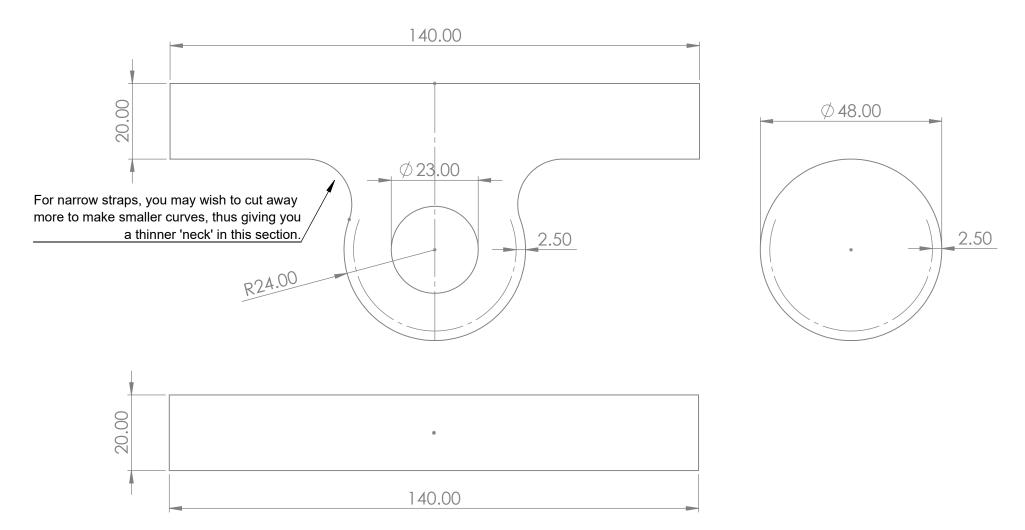
You may wish to make the two straps (currently 140mm) longer if you aim toattach this to a strap or collar wider than 40mm. You can then cut off any excess in the 'fitting' stage.
